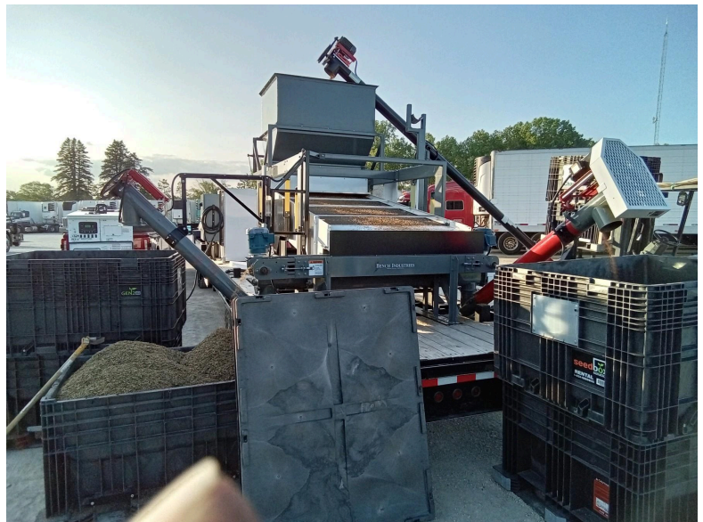
The mobile cleaning unit in operation, with intake and outtake augurs and storage bins. Photo: Paul Novotny
