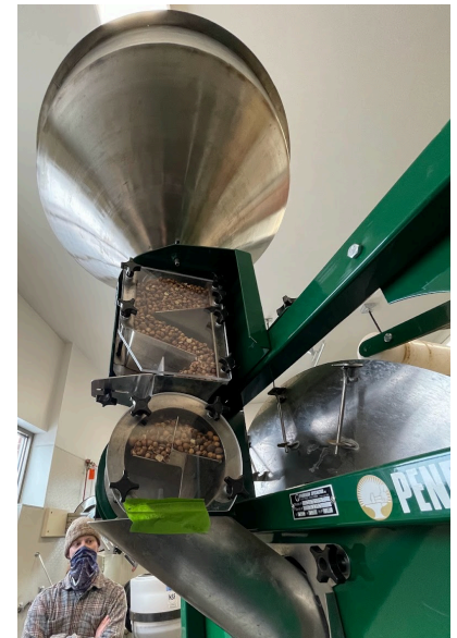
Funneling hazelnuts into the drum sorter at the Ashland processing line. Photo: Emma Dempsey
