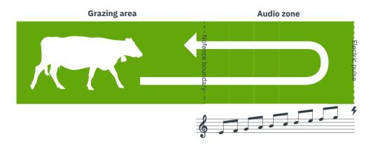
GPS in the collar continuously tracks animal position and checks this against the virtual boundaries set by the producer. As an animal approaches the boundary, a series of audio warnings are delivered. If the animal does not turn away, the collar delivers an electrical pulse.
