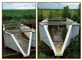
These flumes measure runoff from the STRIPS watersheds. Note the amount of sediment displaced from a 100% no-till crop field (left) compared to a field enhanced with 10% prairie (right).
