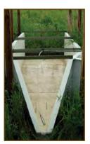
A flume measuring outflow from a 100% prairie field. Note the absence of sediment.
